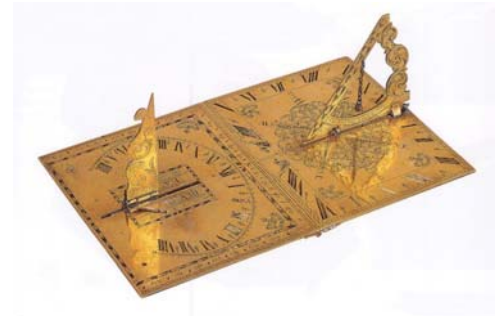
Diagram 4.22: An analemmatic dial which consists of 2 horizontal dials
