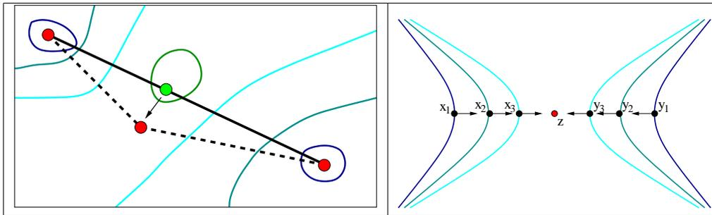
FIGURE 2. The left illustrates path-based methods, and the right illustrates level set methods
