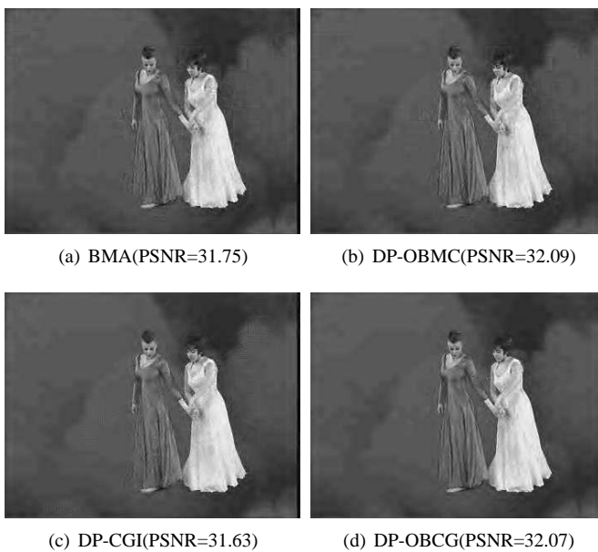
Fig. 10. Perceptual quality of Frame 40 of the Dancer at 230 kbits/sec using various coding techniques.
