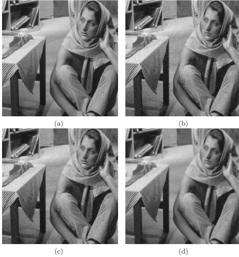
FIG. 3.1. (a) Original image “Barbara”; (b) Noisy image with \sigma = 20 ; (c) Results from MRA framelet; (d) Results from AMRA framelet
